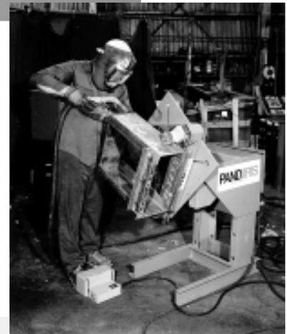
*Positioners provide improved ergonomics as well as optimal welding position in manual welding applications.*
